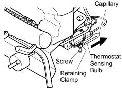
Figure 33 - Removing Thermostat Sensing Bulb
